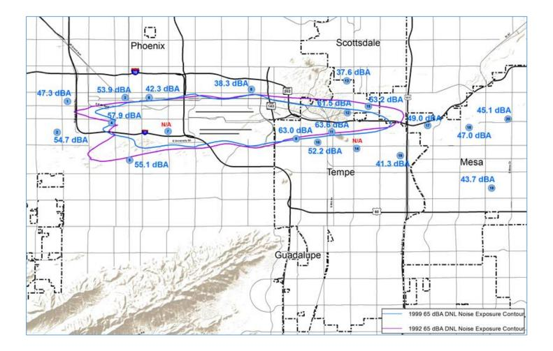
20 noise monitors surround PHX in the communities of Phoenix (8), Tempe (8), and Mesa (4). The noise readings are computed as A-weighted sound level averaged over a 24-hour period with penalty weighting for noise events between 10pm and 7am. Use of the dBA and penalty weighting for nighttime events help ensure noise readings reflect community annoyance factors and issues specific to human hearing and noise energy frequencies.
